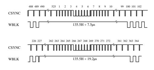
■ H Decoder Pulse Timing Chart for PAL/SECAM
