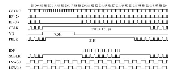
■ Pulse Timing Chart for PAL/SECAM Composite and Vertical Synchronizing Signals (2/2)
